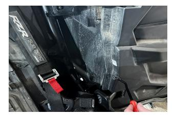
**16. Remove the Door Skin Push Pins (Cont.)** Then remove the (2) push pin located on the bottom edge of the door.
