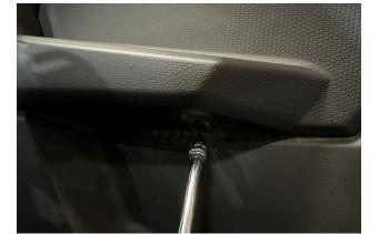
**17. Remove the Door Skin Torx Bolts** Next use a T40 Socket to remove the (1) torx bolt in the middle of the door underneath the armrest.
