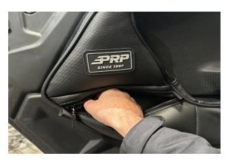
8. Install the Middle and Rear Push Pins Do the same for the middle and rear push pins. Open the pockets, push the pin through the back of the bag, and then all the way into the hole in the door until it is secure.
