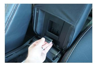
1. Open the Center Console Start by opening the Center Console.
